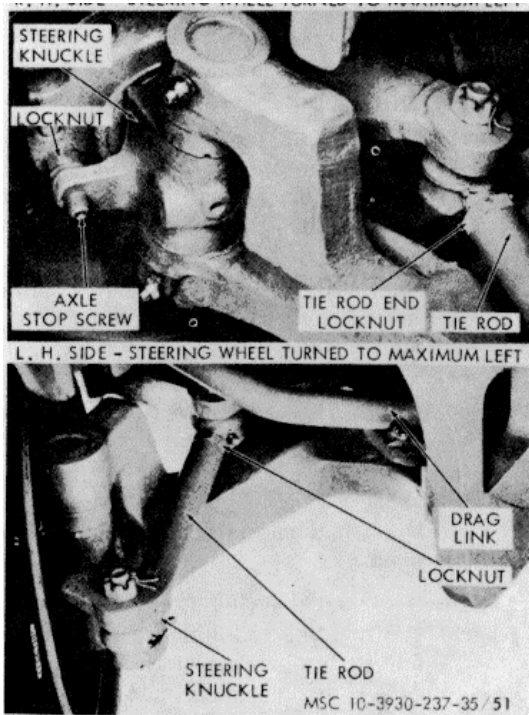
Figure 51. Steering axle and linkage adjustment.
